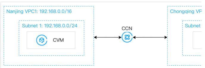
Scenario 2: Multiple VPCs across regions need to be fully interconnected. Since the connectivity of peering connections cannot be transferred, you need to create one peering connection between every two VPCs.
