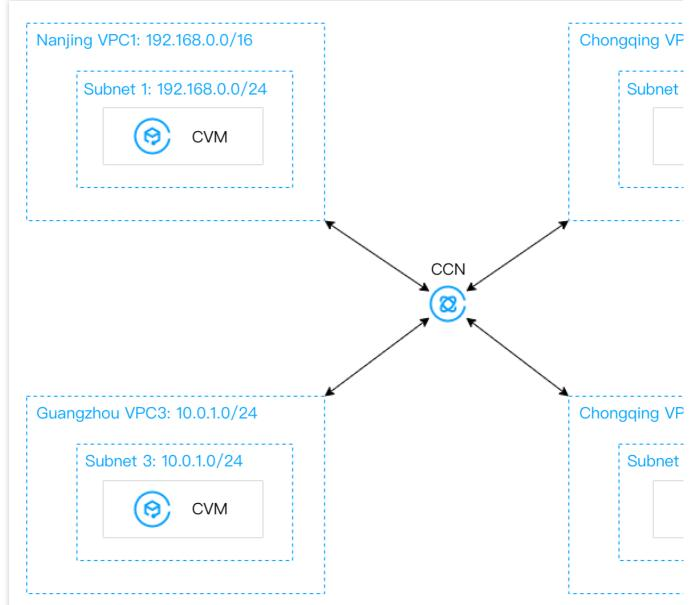
**Scenario 3**: VPC1 is connected to VPC2 and VPC3 respectively through peering connections, but VPC2 and VPC3 are not interconnected.
