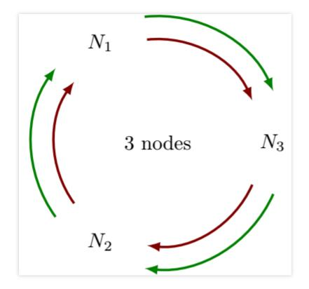
The GM algorithm requires that success be returned only after logs have been synced among all nodes in the cluster, while the Raft algorithm requires sync only among most nodes, which reduces the waiting time in sync route by almost a half.
