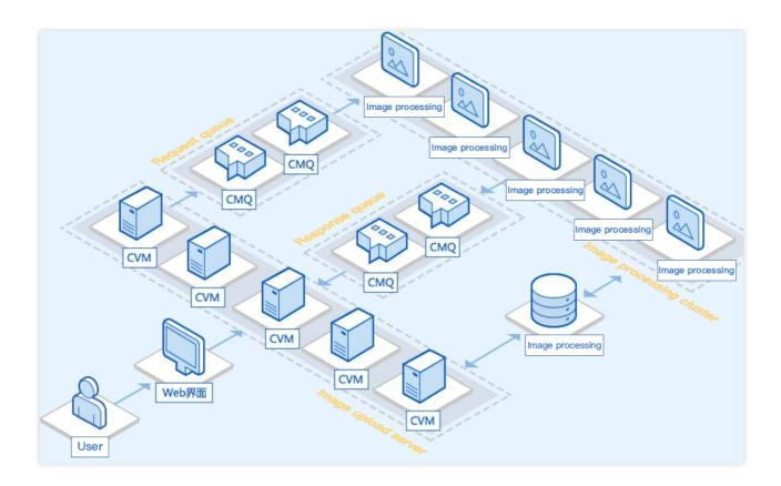
After CMQ is integrated to implement the abovementioned needs, user images will be stored in Tencent Cloud storage (such as CBS and COS), and each user operation request will be stored in the request queue as a message. The message content is an image index composed of elements such as the image name, operation type in user request, and image storage location index key.
