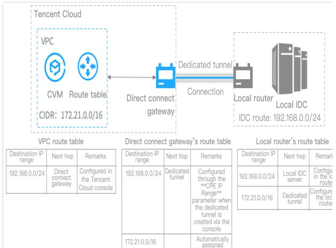
For a BGP dedicated tunnel, the destination IP range of IDC routes to a Tencent Cloud VPC is the VPC CIDR block
