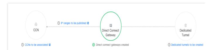
Then the CCN instance will be associated and the CCN icon becomes green. The dotted line between the direct connect gateway and CCN changes to solid, indicating that the interconnection between them is established. 5. Create a dedicated tunnel.
