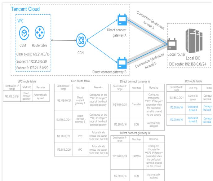
When both dedicated tunnels are BGP, the destination IP range synced from the direct connect gateway A to the local router based on the BGP protocol is the subnet CIDR blocks (172.21.0.0/20, 172.21.16.0/20), while that synced from the direct connect gateway B is the VPC CIDR block (172.21.0.0/16). The route with the longest mask will be matched and used for forwarding. Therefore, the local router will forward all traffic to the direct connect gateway A fails and loses routes.
