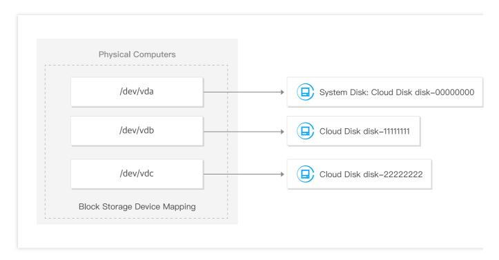
This figure shows how CBS maps the block storage device to the CVM: it maps \dev/vda to the system disk and maps the two data disks to \dev/vdb and \dev/vdc, respectively.
