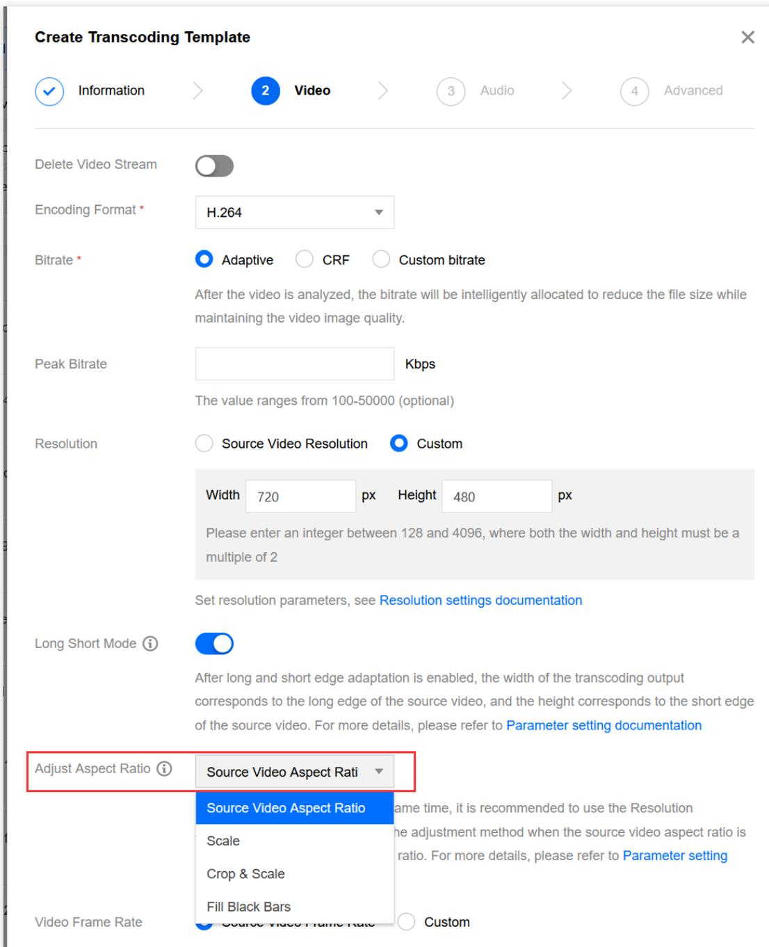
The resolution adjustment methods include maintaining source video aspect ratio, scaling, cropping and scaling, and filling black edges, and their effects are as follows:
